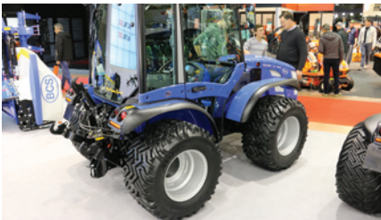
Mitas 440/50R17 IMP AR-04 mounted on the Volcan tractor. These radial traction tyres are ideally suited for working on grassland or on slopes and allow a maximum speed of up to 65 km/h.
